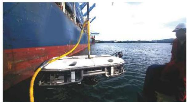
The ROV booster thruster allows cleaning even in strong currents, making it possible to remove barnacle growth up to 50mm thick while working against currents of up to 2 knots.
