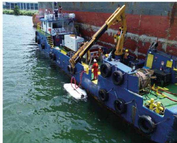
At Balboa, Talleres continues operating the HullWipper ROV, a specialized system designed to "pamper" vessel paintwork by removing slime and grass without damaging coatings.
